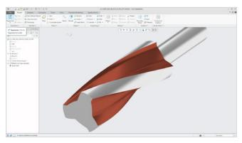
Volume helical sweep – calculate accurate geometry for a Grinding Wheel Scenario.
