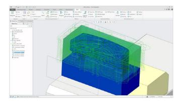
High-speed machining roughing sequence, multi-threaded for fast computation.
