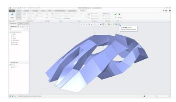
Use box mode to gain a clearer understanding of shapes and enable faster manipulation.
